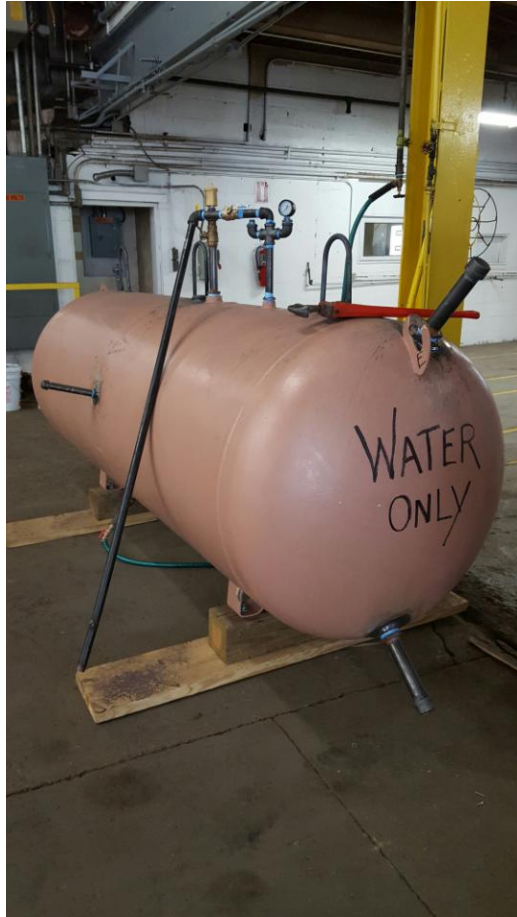
Hydro-Testing After Modification
