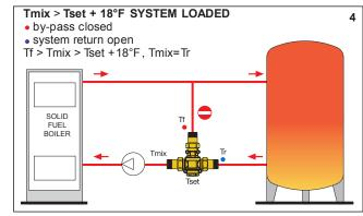
Tmix=Mixed flow to boiler temperature Tr=Return from system temperature
